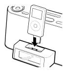
Adjust the rear support forward or backward checking the back of the iPod fits snugly against the rear support to protect the connector
